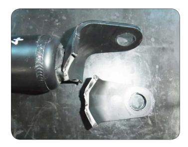
Fatigue test of OME spring seat on weld ring of body assembly tube section. Cyclic loaded 800 kg to 1,500 kg for 500,000 cycles. Sample tested with tooling to represent spring contact on seat. Test represents load at spring length of 305 mm (full extension) to minimum spring length of 190 mm (full compression). No evidence of failure, confirming strength & durability of spring seat internal plate.
